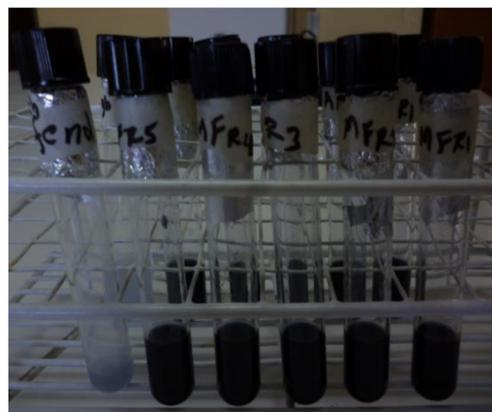
IMAGEN 10: MUESTRAS DESPUÉS DE LA LECTURA DE ABSORBANCIA a 765 nm
