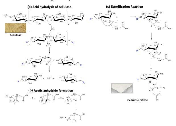
**Figure 2.** (a) Corn husk cellulose and acid hydrolysis reaction, (b) formation of citric anhydride, (c) esterification reaction and cellulose citrate (NCCA).
