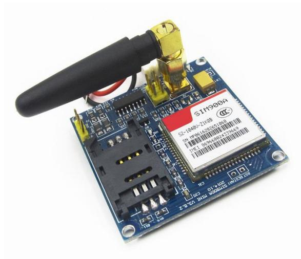
Figura 6. Arduino GSM Shield.
